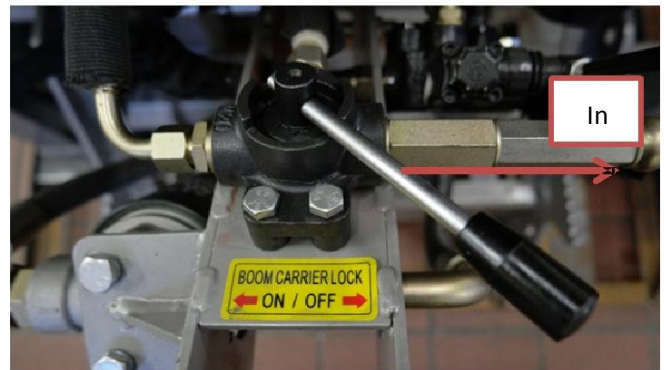
Fig.22 Hydraulic lateral displacement in
