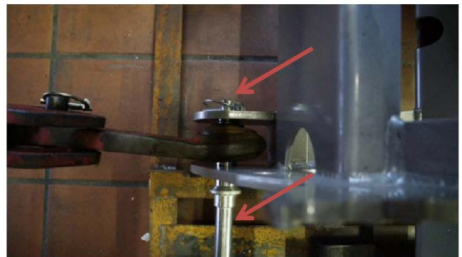
Fig.56 Right side of the lower traverse link secured with bolts and splints
