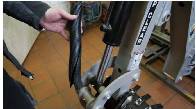
Fig.20 Removing the protective sleeves
