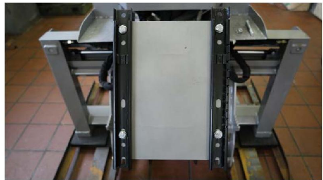
Fig. 34 Bolted on guide rails
