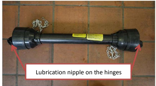
Fig.11 Lubricating the universal joint
