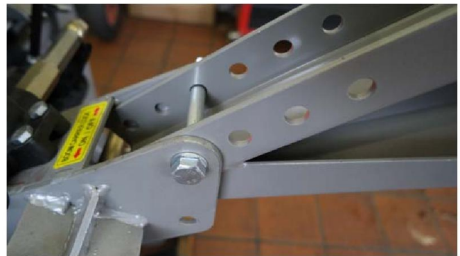
Fig.30 Partially assembled seat rods
