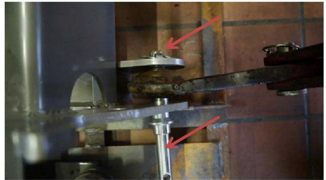
Fig.55 Left side of the lower traverse link secured with bolts and splints
