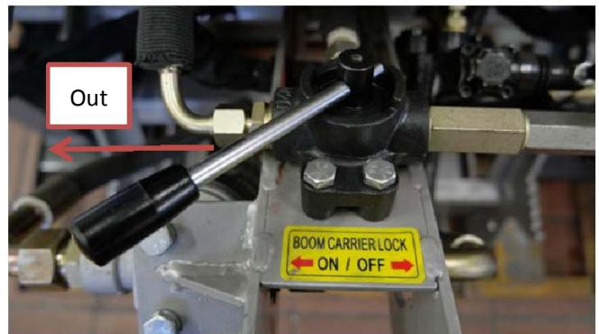
Fig.21 Hydraulic lateral displacement out
