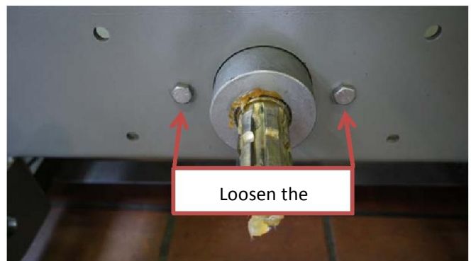
Fig. 13 Hydraulic pump shaft on the digger
