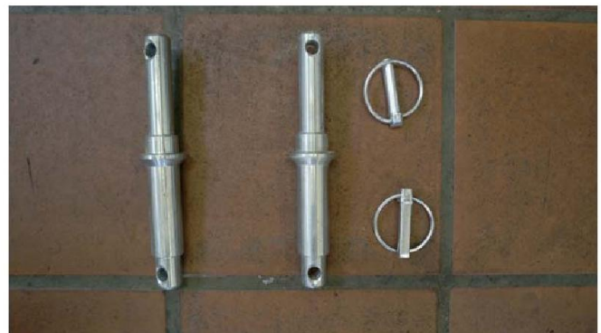
Fig. 53 Bolts and splints for lower link
