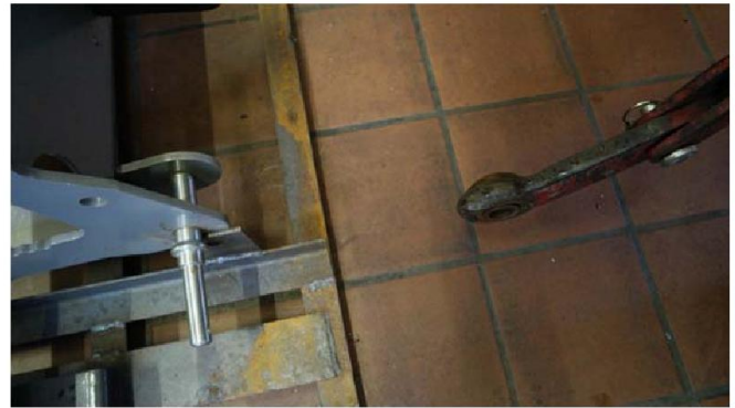
Fig. 54 Bolts and lower traverse link
